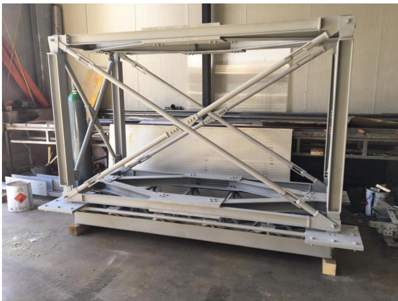
Figure 1. Dual steel frame (DSF) with a new brace-type damper made of a shape memory alloy material.
