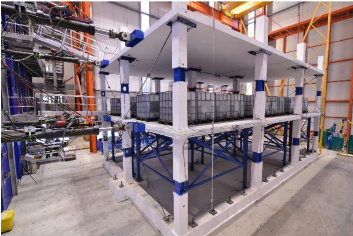
Figure 2. Test specimen: a two-storey flat slab structure
