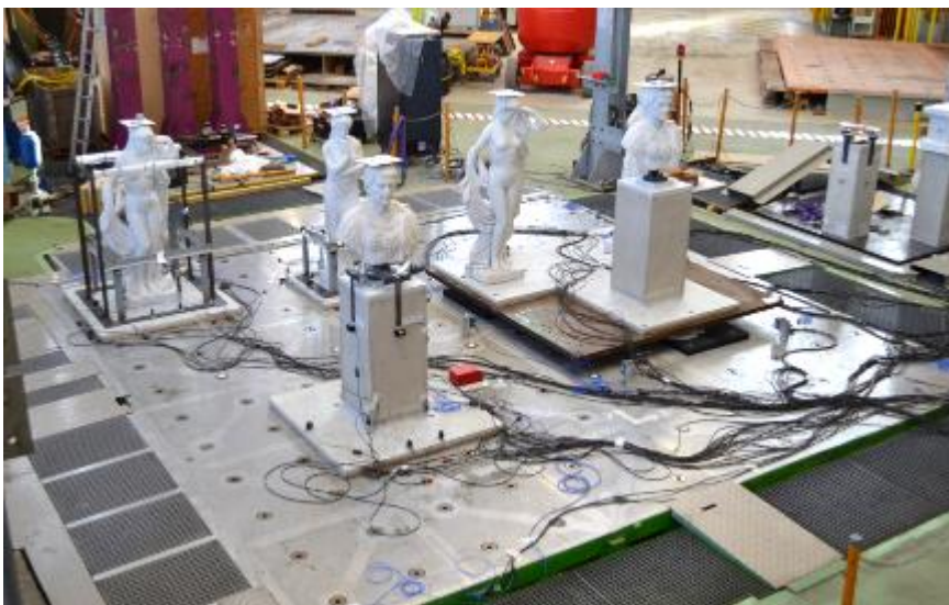
Figure 3. General set up of the statues and busts on the shake table
