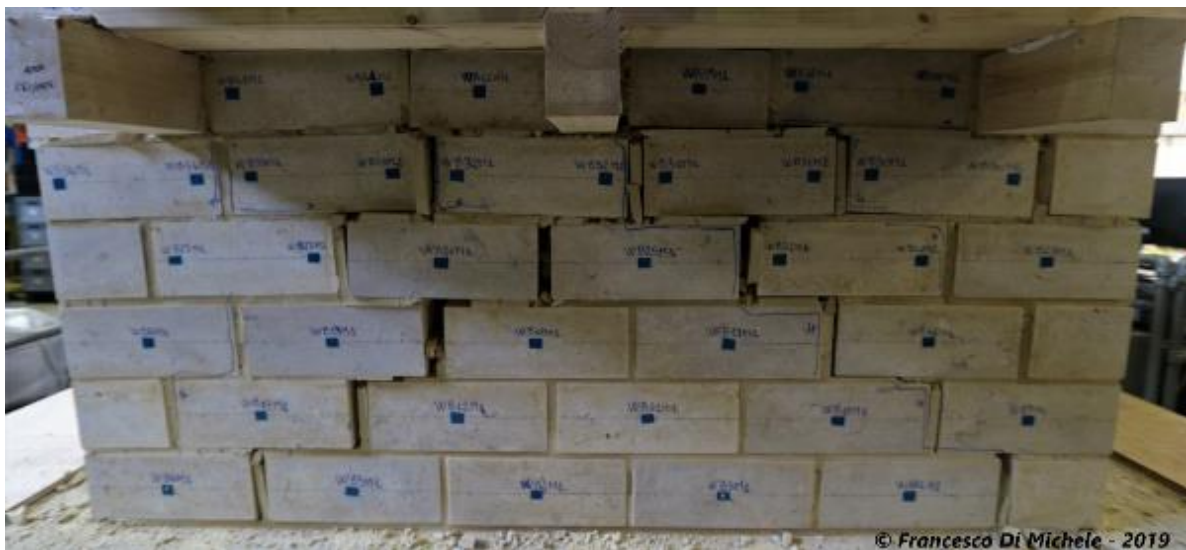
Figure 1. Typical masonry wall specimen tested.
