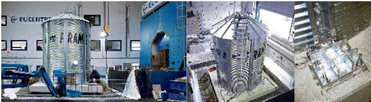
Figure 1. Full-scale silo structure tested in as-built and seismic isolated configurations
