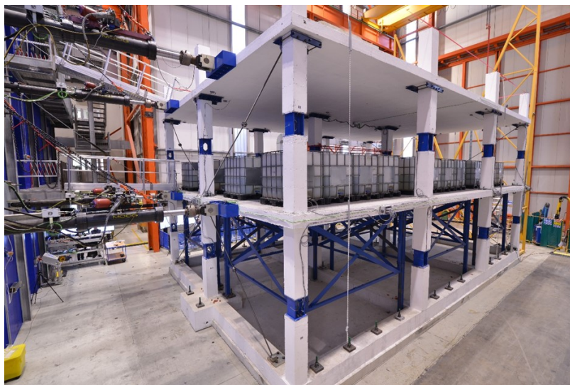
Fig. 1: The full-scale two-storey test specimen as flat slab structure
