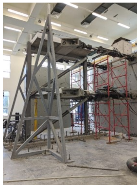
Fig. 3: Three-dimensional (left) and two-dimensional (right) multi-storey 2/3 scaled steel frames tested with the PsD method using the advanced facilities of the StruLab of University of Patras, Greece
