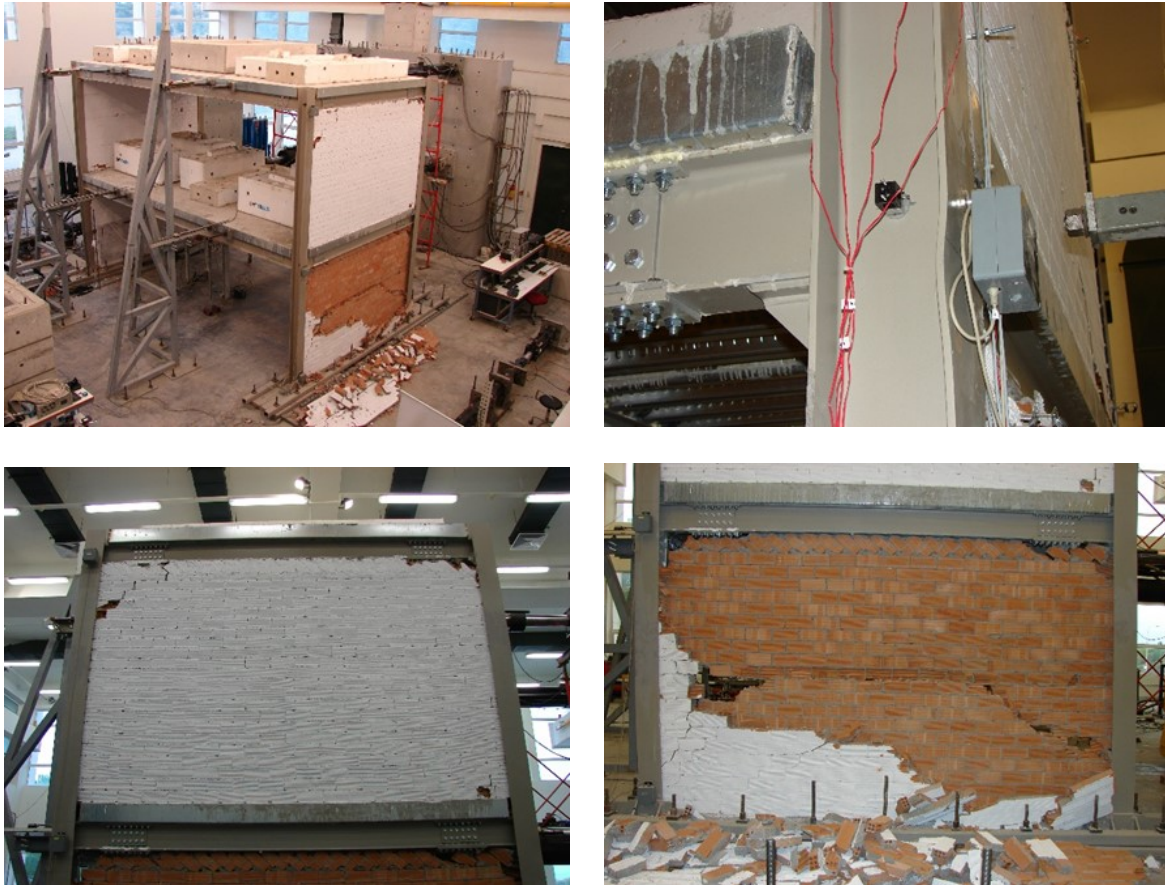
Fig. 4: Observed damage on the 3D steel frame after the Norcia earthquake sequence with a scaling factor of 3.0
