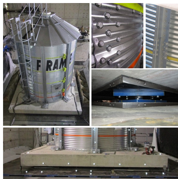
Fig. 1: The flat-bottom cylindrical silo on the shake-table
